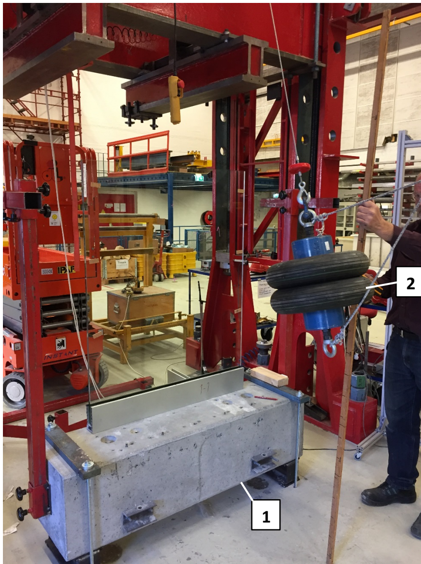
Figure 6. Applied test setup for pendulum test.
