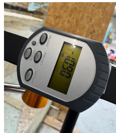
Digital dial indicator (accuracy 0,01mm)
