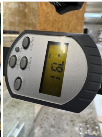
Digital dial indicator (accuracy 0,01mm)
