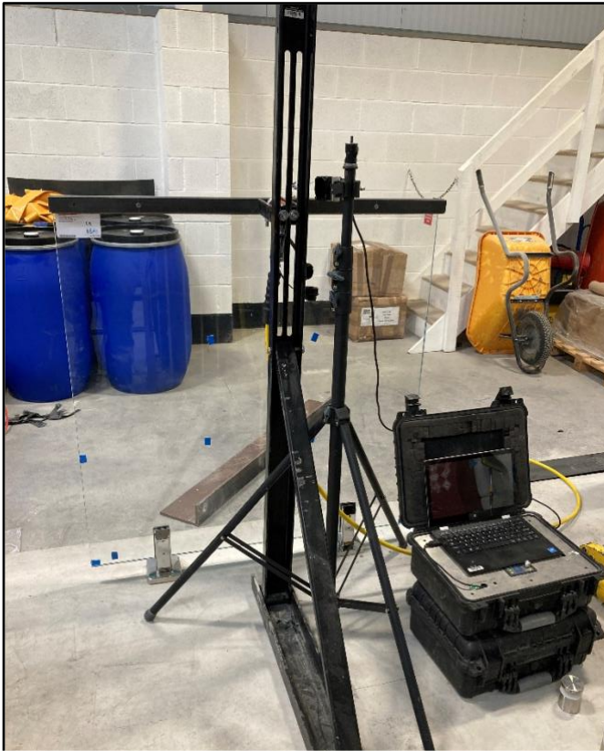
Photographs 1&2 – Photograph 1 shows the equipment and method of the uniformly distributed line load testing. Photograph 2 shows the equipment and method of the 1m 2 Infill load testing.
