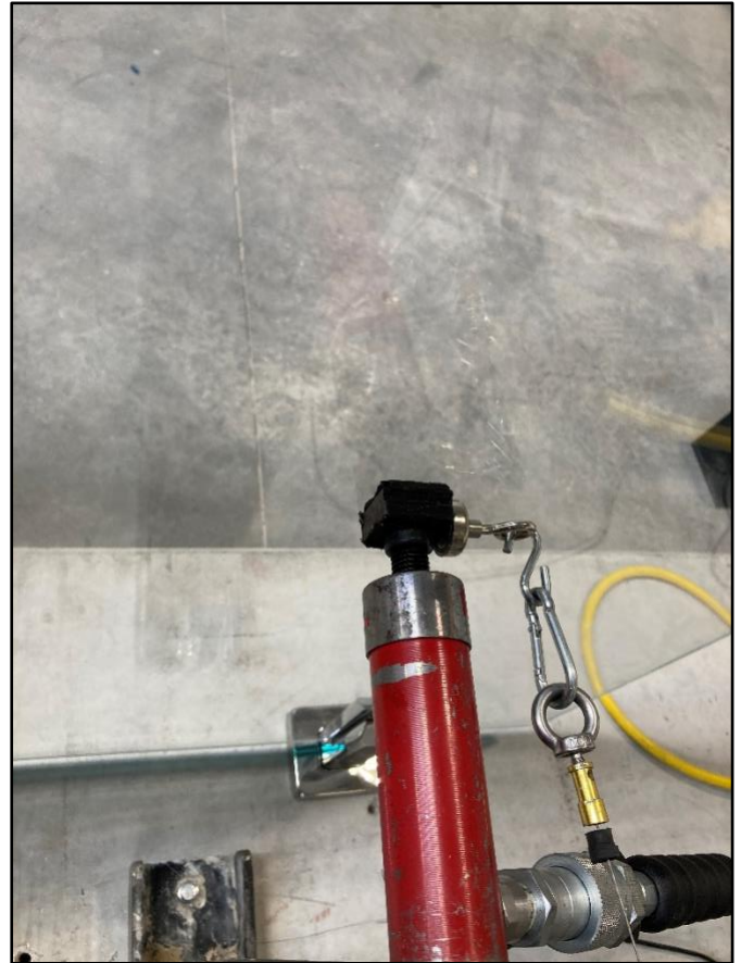
Photographs 3&4 – Photographs 3&4 shows the equipment and method of the point load testing.
