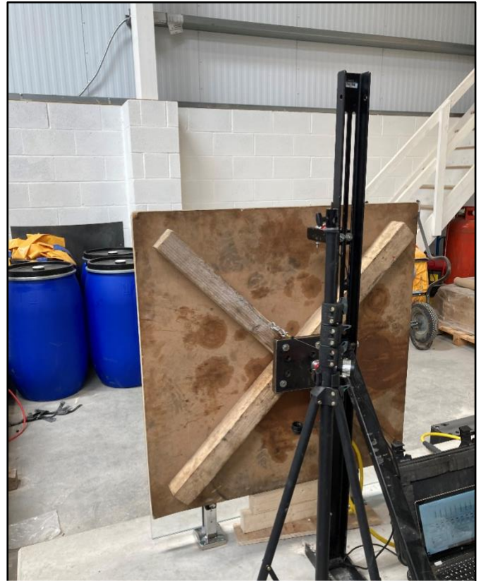
Photographs 1&2 – Photograph 1 shows the equipment and method of the uniformly distributed line load testing. Photograph 2 shows the equipment and method of the 1m 2 Infill load testing.
